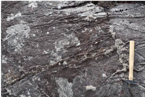
Figure Cuillin 7.19: Hornfelsed basaltic lava on the west side of the Abhainn Camas Fhionnairigh, c. 60m above the level of the river, with abundant veins containing various secondary hydrothermal minerals, including epidote, chlorite, various zeolites and carbonates. Hammer c. 30cm long.
