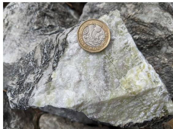
Figure Strath 2.15: Typical fresh surface of marble, with distinctive yellow-green serpentine after forsterite. Coin c. 24mm across.
