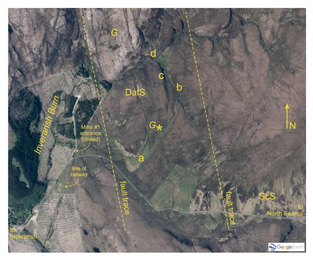
Figure 11-26 – Annotated Google Earth<sup>®</sup> image of the opencast area (a, b, c & d) and Mine #1 entrance in the vicinity of the Inverarish Burn.
