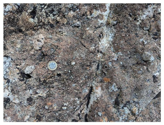
Figure 5-70 – Typical coarse volcaniclastic breccia from the Srath na Crèitheach area, SE of Meall Dearg. Coin c. 24mm across.
