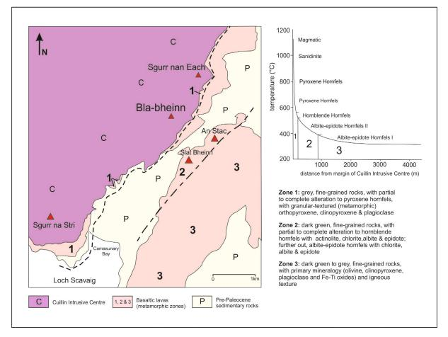
Figure 6-49 – Zones of thermal alteration within the basaltic lavas on Strathaird and south of Sgùrr na Stri (after Almond 1964).
