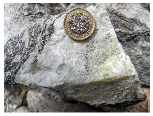
Figure 11-1 – Typical marble from one of the abandoned quarries at Kilchrist. The green coloration is metamorphic olivine replaced by secondary serpentine. Coin *c.* 24mm across.
