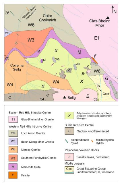
Figure 5-78 – Geological map of the Belig area illustrating the distribution of the breccias.
