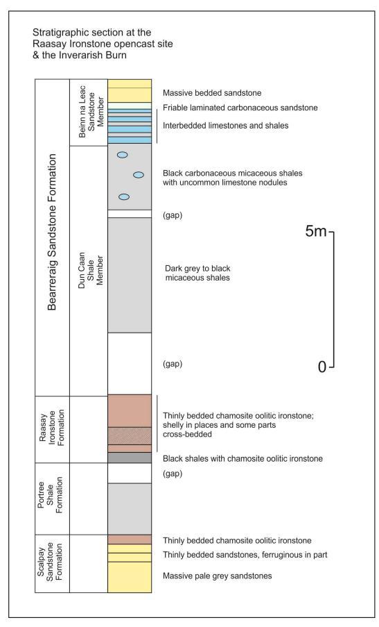
Figure 11-23 – Details of the stratigraphy of the Raasay Ironstone Formation, together with underlying and overlying strata.
