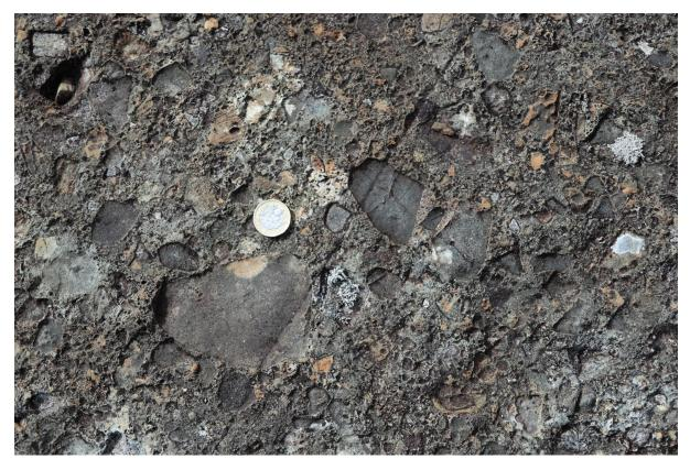
Figure 5-69 – Typical coarse volcaniclastic breccia from the Srath na Crèitheach area, SE of Meall Dearg. Coin c. 24mm across.
