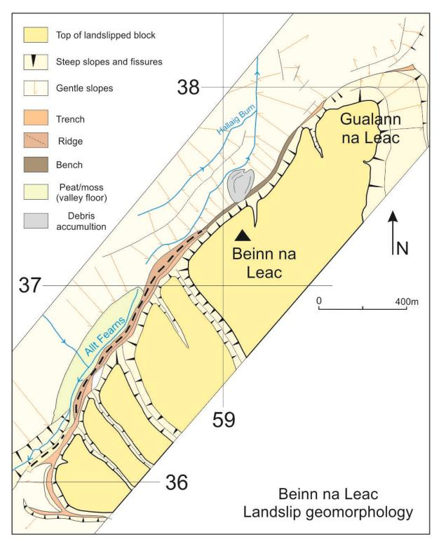
Figure 10-61 – Details of geomorphological features associated with the Beinn na Leac Landslip (after Smith et al. 2009, who refer to it as the Hallaig Landslip).
