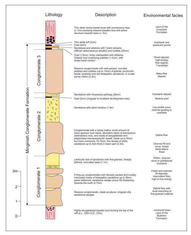
Figure 5-38 – Stratigraphical section for the Allt Geodh a' Ghàmhna Member of the Minginish Conglomerate Formation (based on Williamson & Bell 1994).
