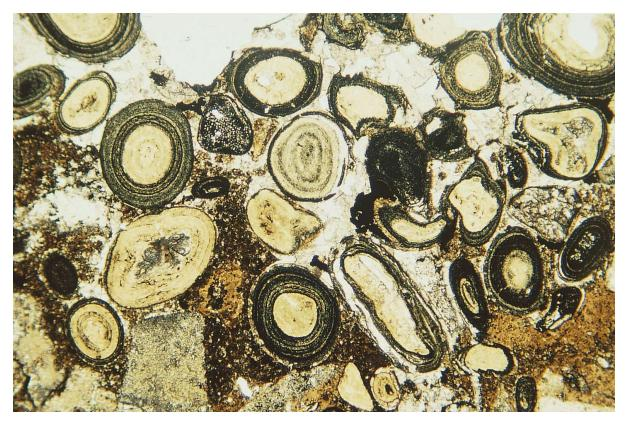
Figure 11-24 – Photomicrograph of the Raasay Ironstone Formation chamositic ooidal ironstone with echinoderm fragments in a carbonate matrix/cement. Image *c.* 5mm across. View under plane polarised light.
