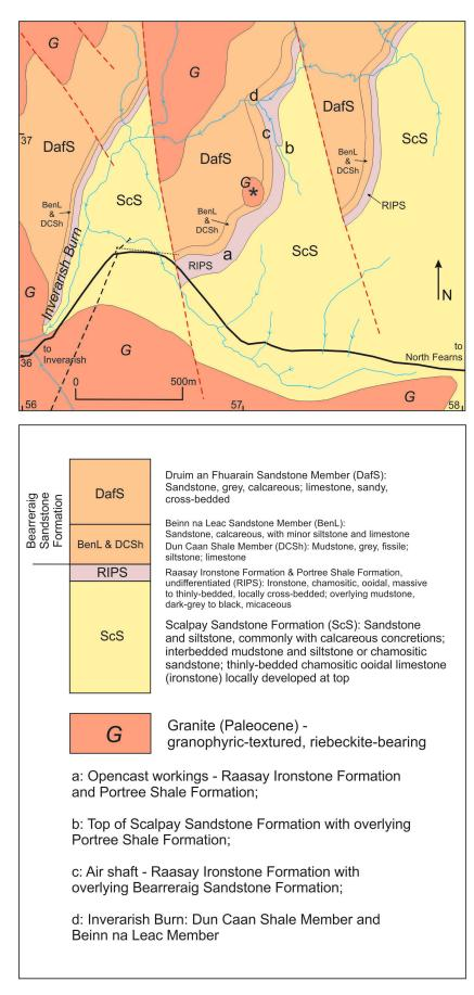
Figure 11-25 – Simplified geological map and stratigraphic details of the opencast area and mine in the vicinity of the Inverarish Burn.
