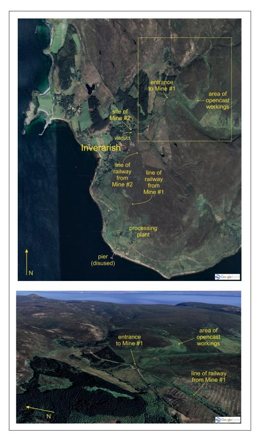
Figure 11-27 – Annotated vertical and oblique Google Earth<sup>®</sup> images of the area involved in the exploitation of the Raasay Ironstone Formation, including the opencast area and Mine #1 in the vicinity of the Inverarish Burn.
