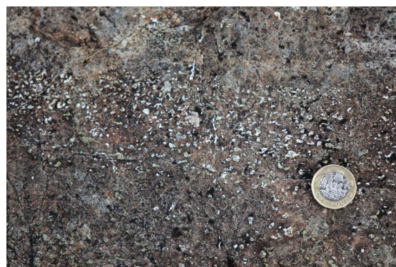
Figure Red Hills 4.10: Hornfelsed amygdaloidal basalt lava, Glen Sligachan. Coin c. 24mm across.
