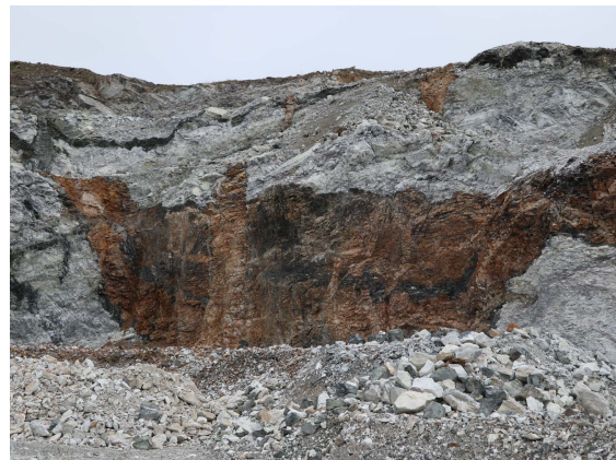
Figure Strath 3.31: Detail of the Torrin Quarry, with dark Paleocene dolerite dykes intruded into pale Cambro-Ordovician Durness Group dolostones.
