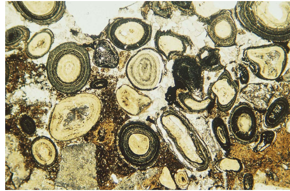
Figure Raasay 4.3: Photomicrograph of the Raasay Ironstone Formation chamositic ooidal ironstone with echinoderm fragments in a carbonate matrix. Image c. 5mm across. View is under plane polarised light.
